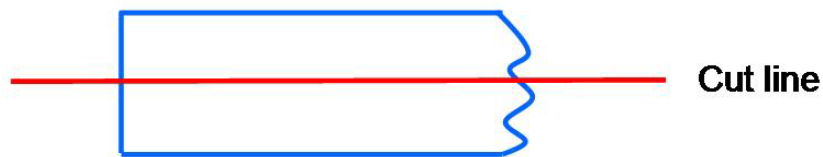
Figure 3.10 Cut line for cross-sectioning of creep fracture specimens
