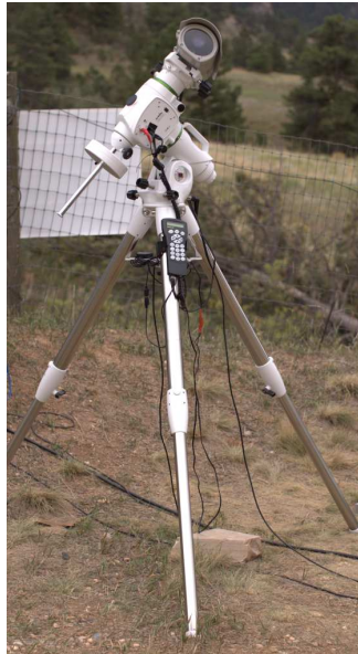
Figure 2.2: SatNOGS Optical ground station prototype.
