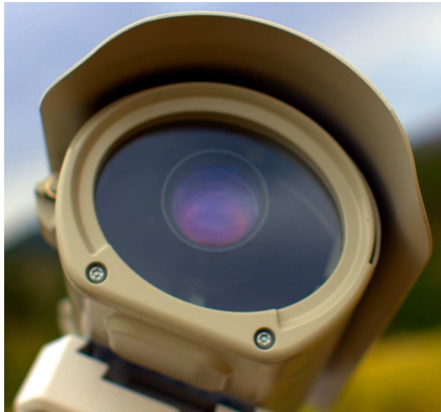
Figure 3.2: Camera enclosure, front side, showing glass and lens.
