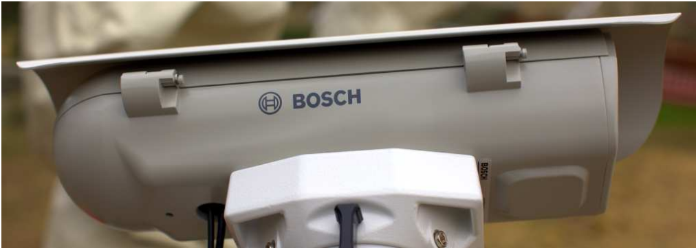
Figure 3.3: Camera enclosure, left side, showing hinge.
