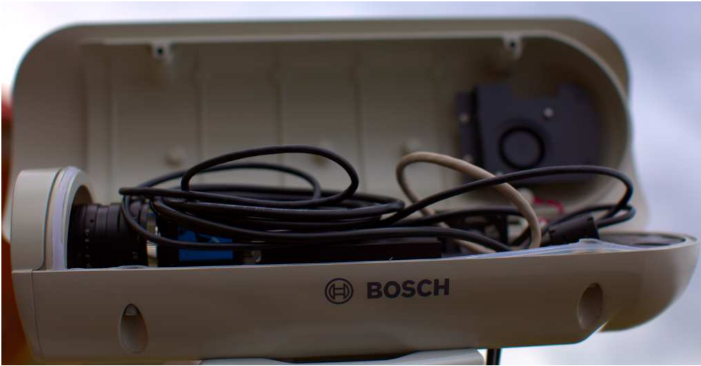
Figure 3.5: Camera enclosure, right side, opened.
