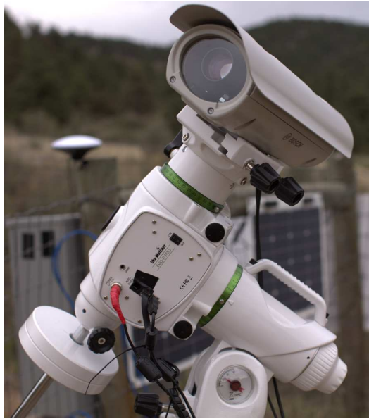
Figure 3.1: SatNOGS Optical ground station prototype.
