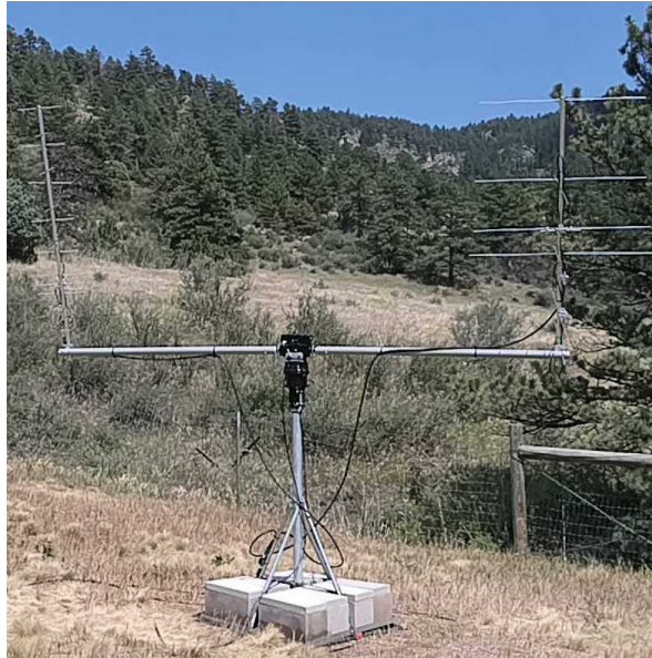
Figure 2.1: SatNOGS ground station with antennas.
