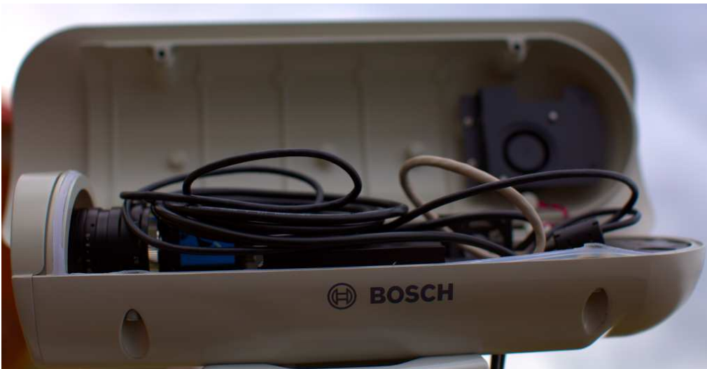
Figure 3.5: Camera enclosure, right side, opened.
