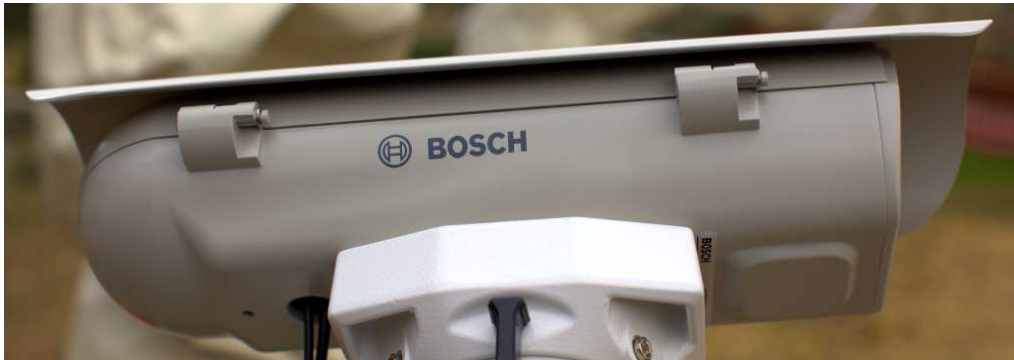
Figure 3.3: Camera enclosure, left side, showing hinge.
