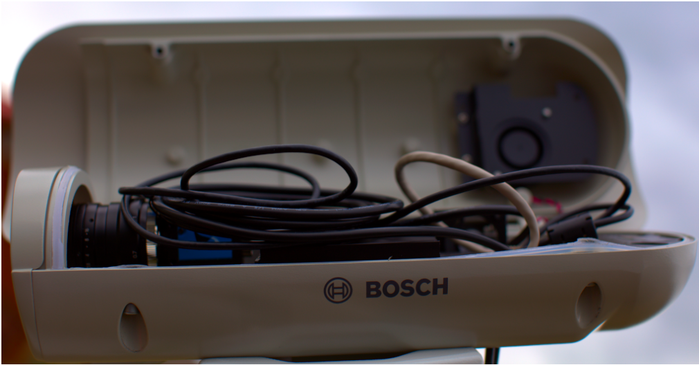
Figure 4.5: Camera enclosure, right side, opened.
