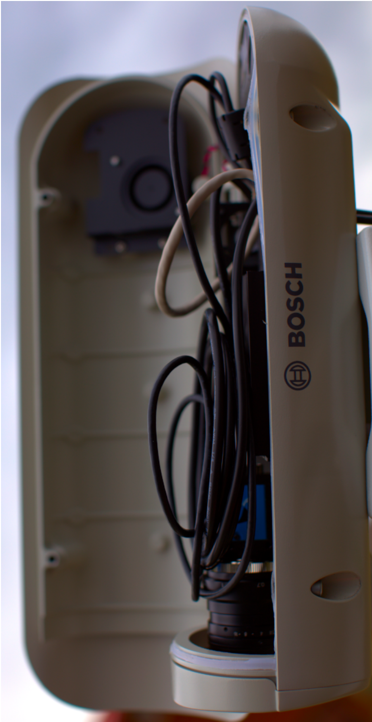
Figure 4.5: Camera enclosure, right side, opened.
