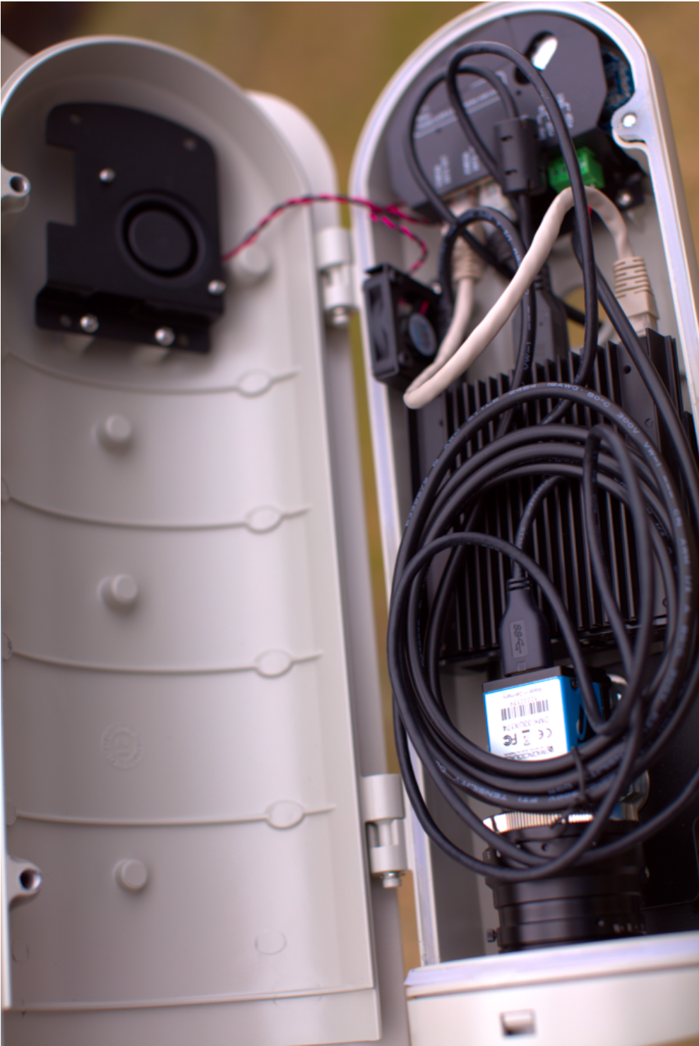
Figure 4.6: Camera enclosure, opened.
