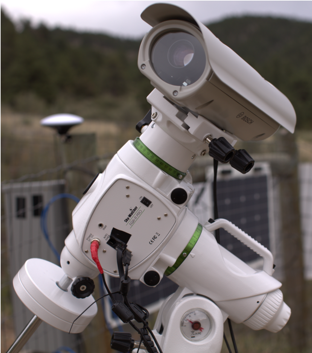
Figure 4.1: SatNOGS-Optical ground station prototype.
