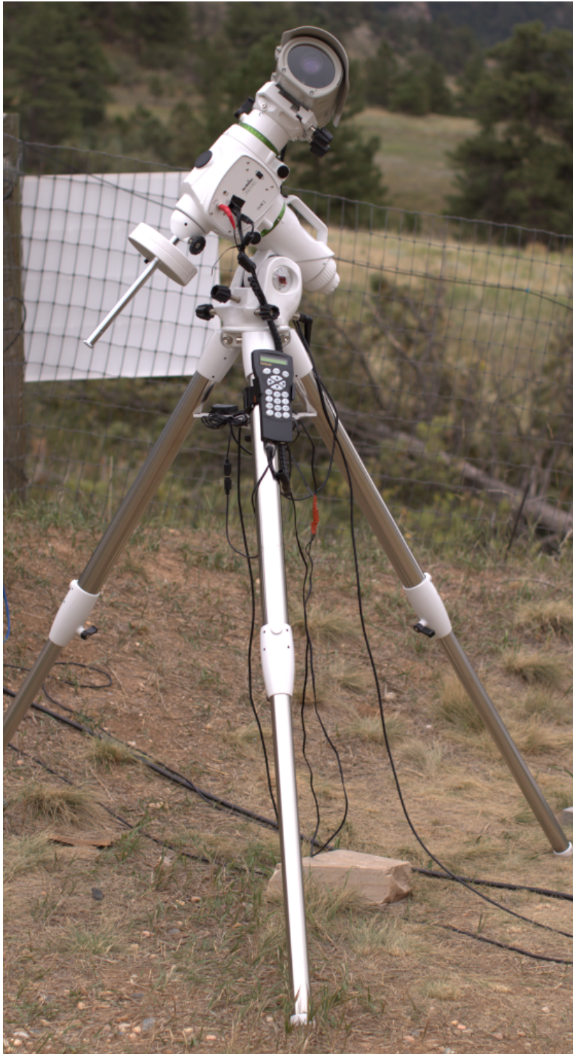
Figure 2.3: SatNOGS Optical ground station prototype.
