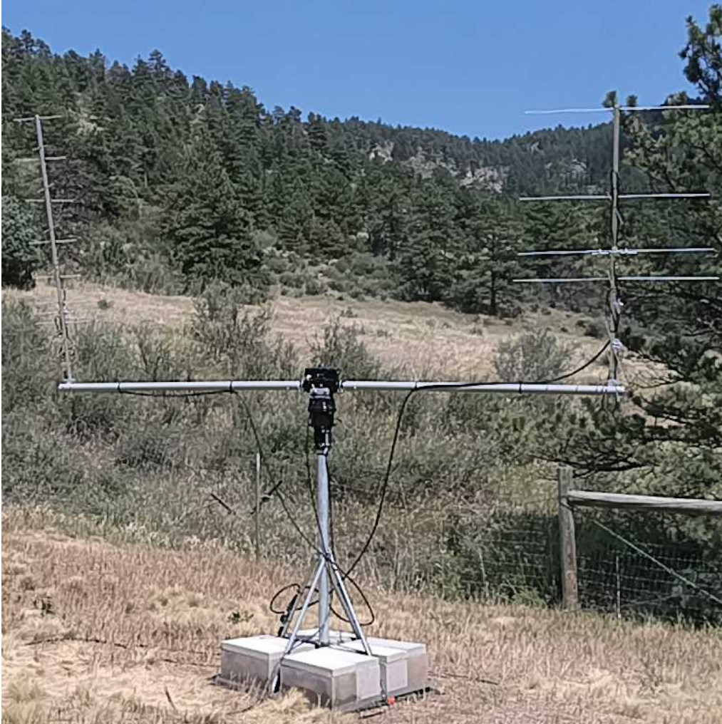
Figure 2.1: SatNOGS ground station with antennas.
