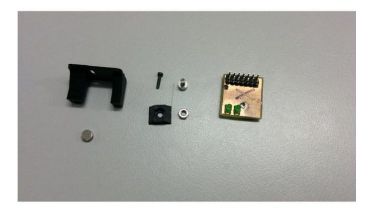
Place the nut into the 3D printed part
