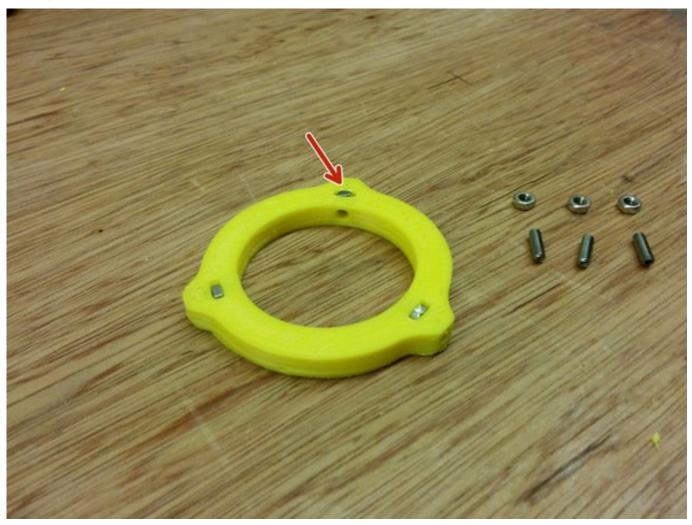
Insert the nuts in the pockets of 3d printed part, then screw the set screws as shown.
