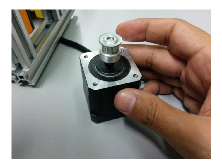
Place the motor under the mount and tighten the screws.
