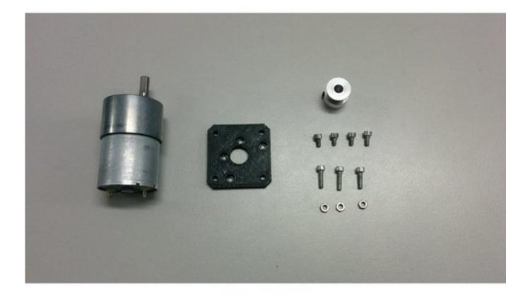
Bolt the motor on the flange
