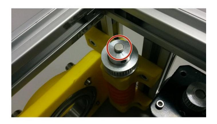
Bolt and align the encoder over the magnet using the M3 screw
