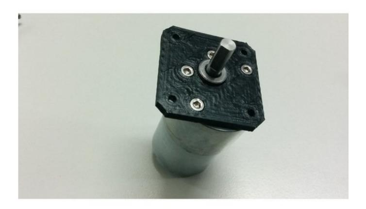
Insert the small pulley over the motor shaft and the larger through the worm shaft. Bolt the flange, with the motor, on the motor base.
