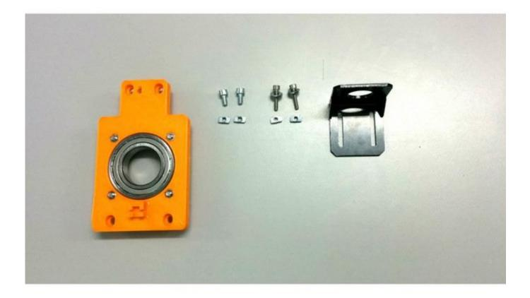
Attach the bolts, slot 6 nuts and the stepper motor mount. Finally attach the whole assembly to the frame.
