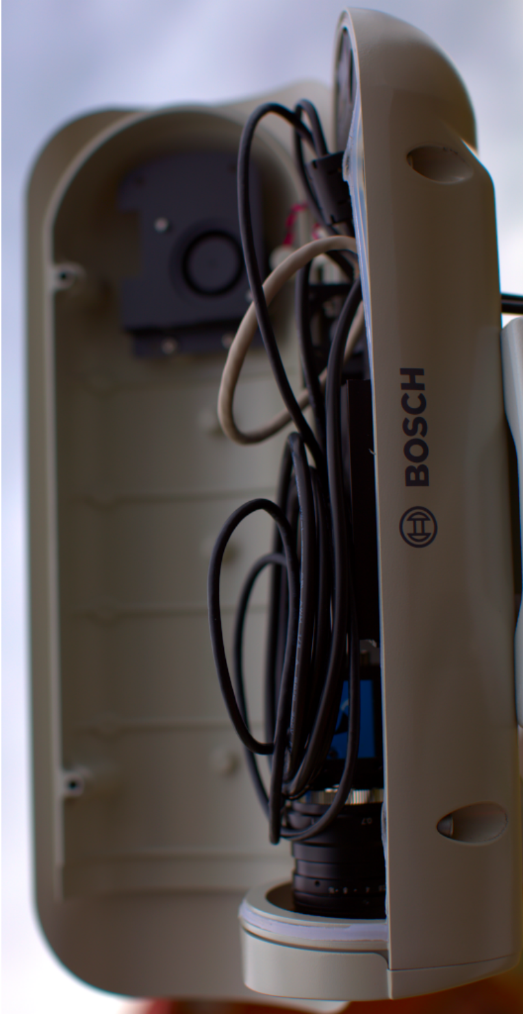
Figure 4.5: Camera enclosure, right side, opened.
