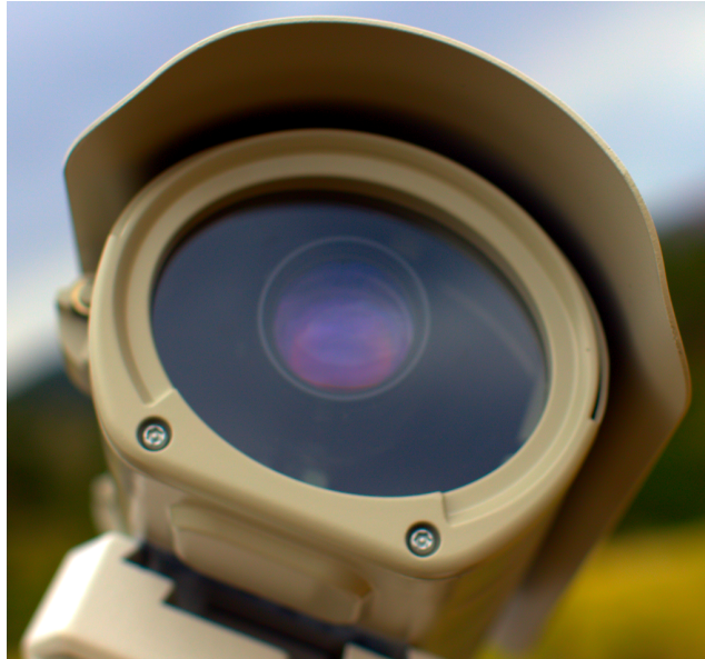
Figure 4.2: Camera enclosure, front side, showing glass and lens.
